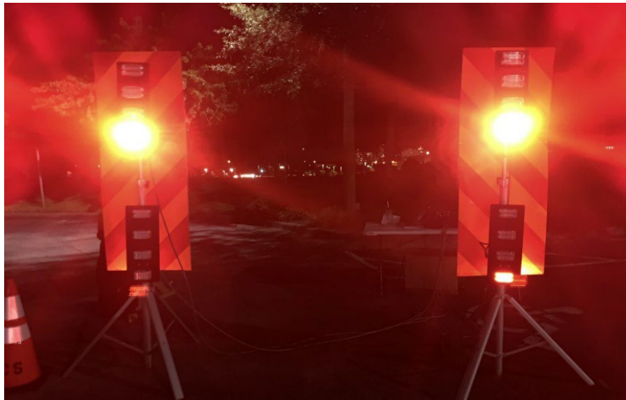
Figure 3. Mounting configuration for the flashing emergency lights used in the study; also shown are reflective marking panels behind each set of lights.
